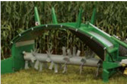
The solid arch construction made of 6 mm steel ensures a very high stability.
