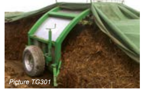
The fabric cover is joined to a smaller width to allow gases to escape. The hard manual work involving the wet fabric is avoided.
