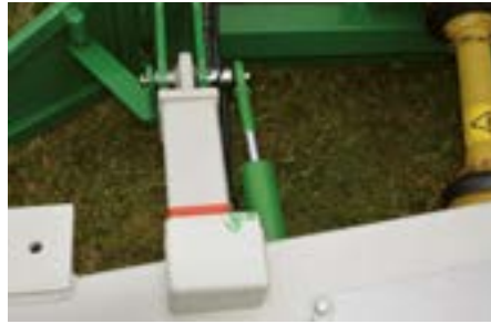
Hydraulic tilting system of the tunnel, so that the battery stays in the site where it belongs.
